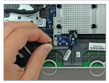
Disconnect the IR board cable by pulling its connector toward the left edge of your iMac.
