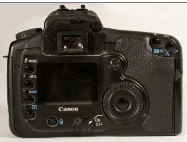
Pull up on both sides of the the eyepiece cap. It should come off with little pressure.
