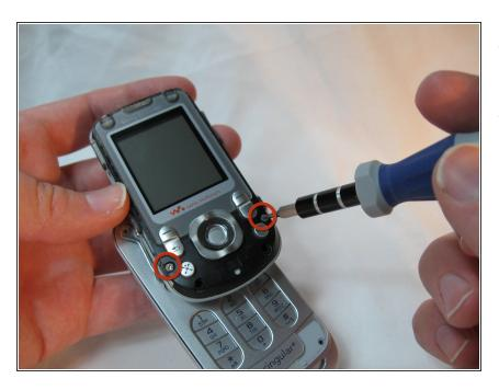
Remove the Torx screws near the buttons.
