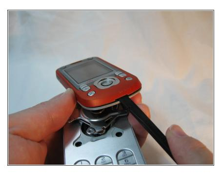
Gently pry off the front face, starting at the bottom slot.
