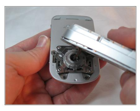
The back housing is now disassembled, and the swivel assembly is revealed.
