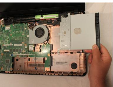
Gently slide the CD drive away and pull up to remove it from the computer.
