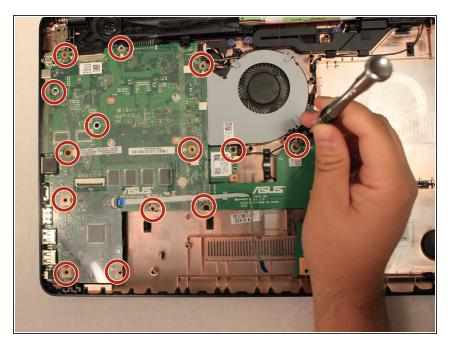
Remove all fourteen 4.3 mm screws from the motherboard. Use a Phillips #1 screwdriver to remove the screws.
