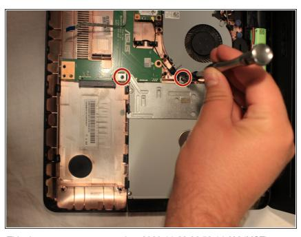
Remove the three 5.7 mm screws from the CD drive mounting points.
