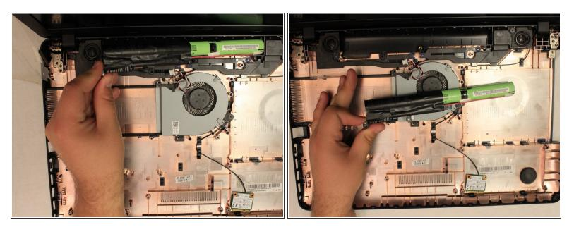
• Pull up on the left side of the battery at an angle to pry it out of the battery slot. Note that the battery will have originally been glued down and may be difficult to get out.
