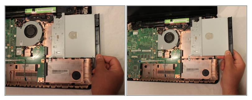
• Gently slide the CD drive away and pull up to remove it from the computer.
