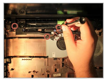
Remove the three 4.3 mm screws holding the battery pack with a Phillips #1 screwdriver.
