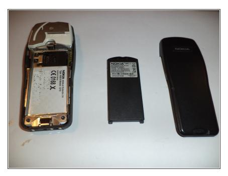
Remove Battery cover, battery and SIM Card.
