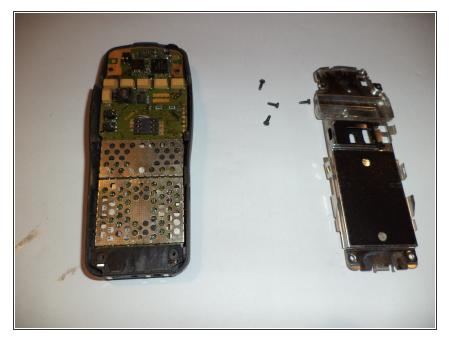
If you remove the plate, you can see the Motherboard. Remove the Motherboard with a small flathead screwdriver or a spudger. (A spudger is recommended).
