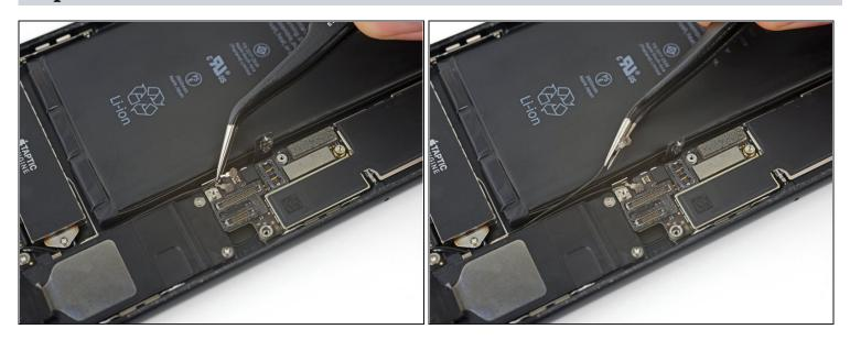
Carefully de-route the coaxial cable you just disconnected from the small metal clip holding it to the logic board.
