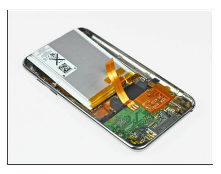
Flip your battery over and lay it down in the rear panel as shown.
