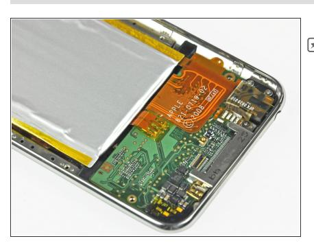
Don't forget to reapply the piece of tape over the solder pads to prevent any shorts.
