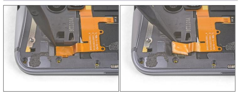
• Use the tip of a spudger against the corner of the flash connector to pry the connecter straight up and out of its socket.
