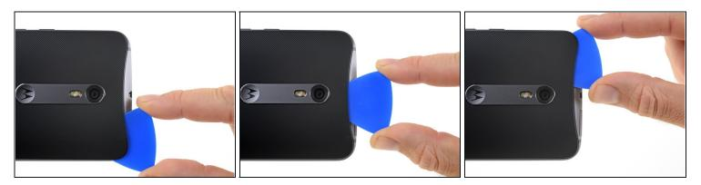
• Slice through the adhesive along the top edge of the phone, pulling the pick out slightly to guide it around the rear-facing camera.
