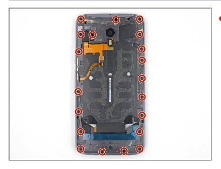
• Use a T3 Torx driver to remove twenty 2.4 mm screws.
