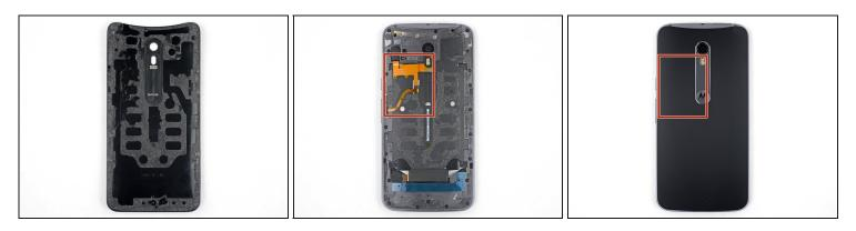
• In the following steps, you'll be cutting through the adhesive securing the back cover.
