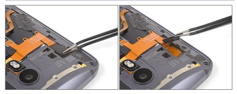
• Use tweezers to lift away the rubber cover over the flash connector.
