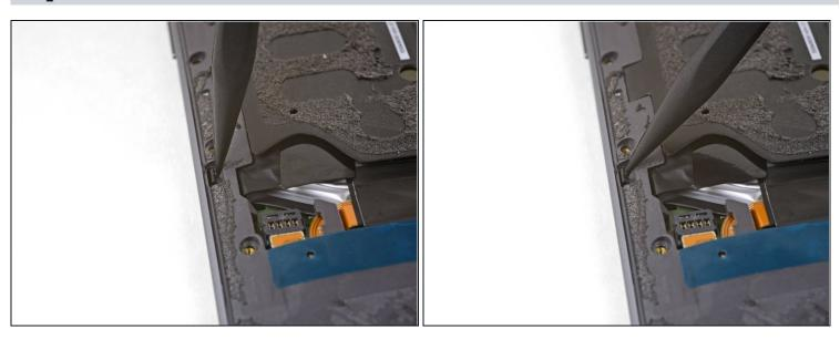
• Use the point of a spudger to push the small clip securing the left side of the midframe toward the edge of the phone, releasing the clip.
