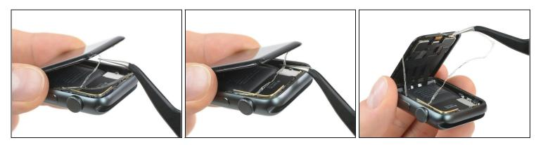
To avoid straining the display cables, don't open the display all the way yet.
