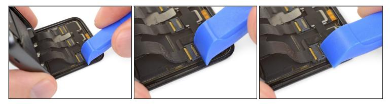
• Carefully use a pry tool or a clean fingernail to unlock the first of the three **ZIF** connectors by prying up the small black locking flap opposite the cable.
