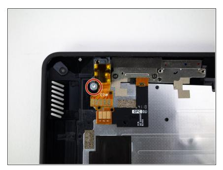
Remove the single 3.1mm T5 Torx screw from the headphone jack.
