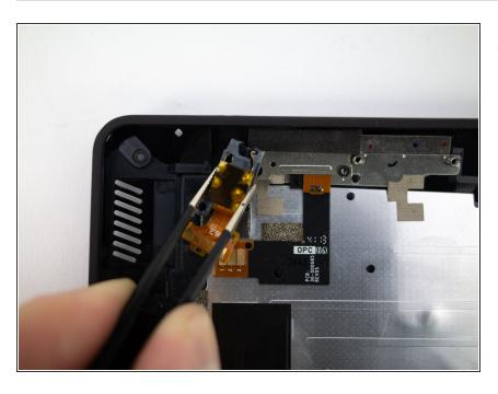
Pull the headphone jack out of its socket with a pair of tweezers to remove.
