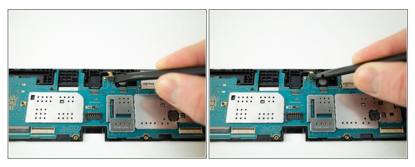
Use the flat end of a spudger to disconnect the IR sensor press-fit connector from the motherboard.
