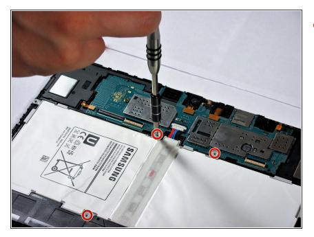
• Use a Phillips #00 screwdriver to remove the four 3.2mm screws.
