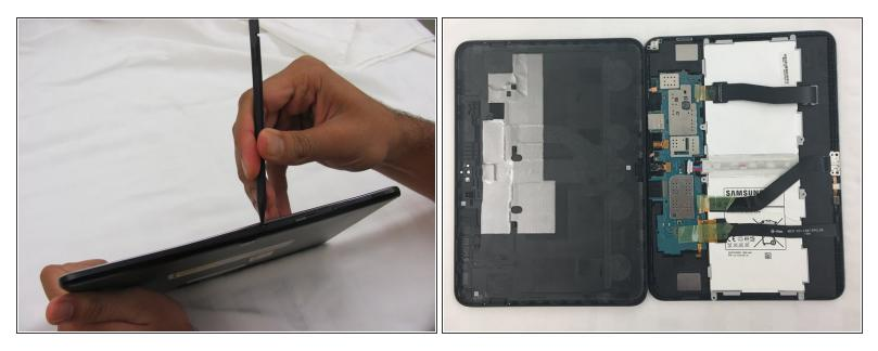
Insert the wedge of the nylon spudger and slide it between the front and back panels until the back comes off.
