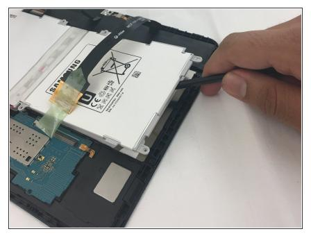
• Use the nylon spudger to remove the battery by prying up on the edges.
