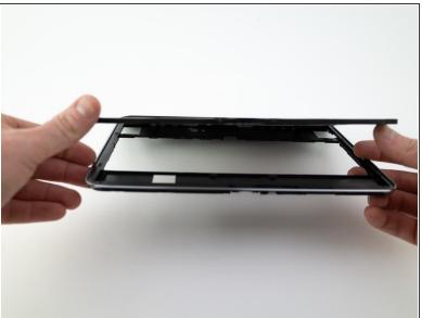
Hold the frame with both hands and push the LCD display up from underneath with your fingers.
