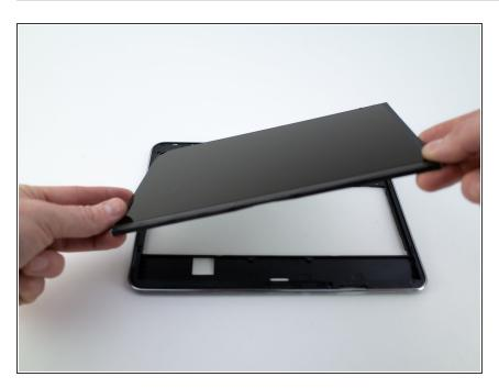
Remove the LCD display.
