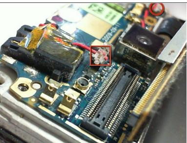
Locate the two wired connections on the top circuit board.
