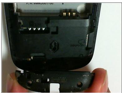
Pull out the antenna cover to access the motherboard.
