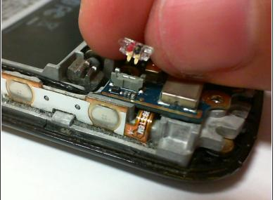
Remove the wired connections by using a squeeze-and-pull action.
