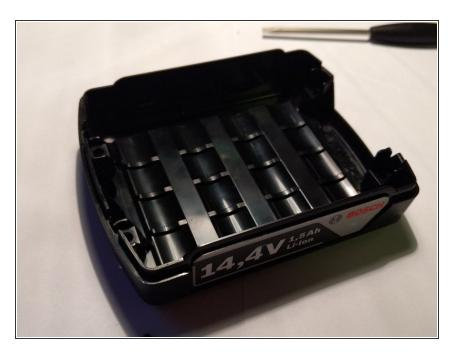
Lower lid hides no surprises, just ergonomically shaped bottom which holds the li-ion cells nicely fit in place.
