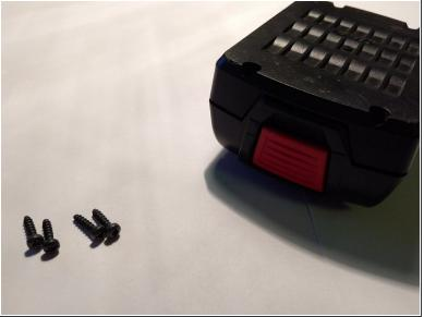
Bosch battery is held together by 4 combo screws, which will fit both flat and torx screwdrivers.
