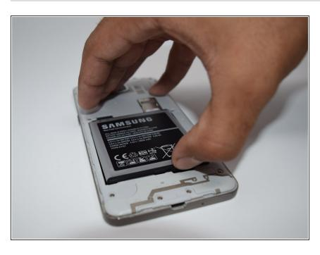
To remove the battery, lift up on the thumb tab located on the bottom right corner of battery bay.
