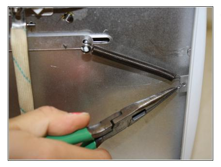
Use pliers to bend the spring back into place if necessary.
