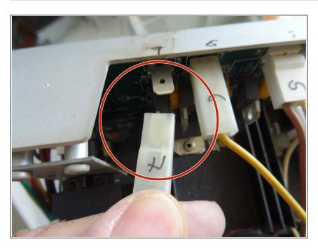
The blue cable from the thermoblock leads to the connector on the electronics, which is marked with 7
