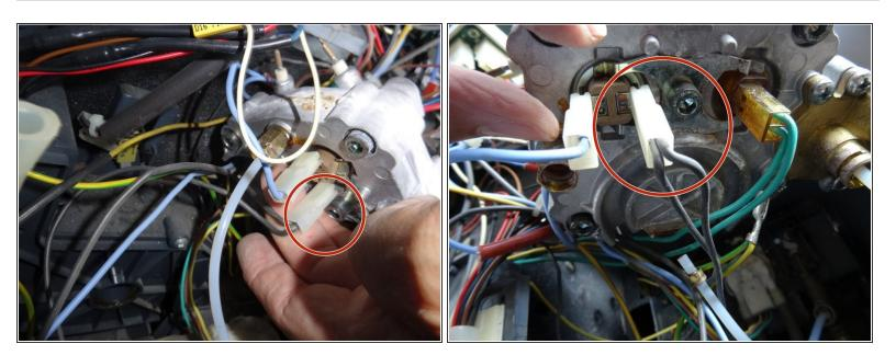
Disconnect the connector with the two gray cables from the thermal switch.
