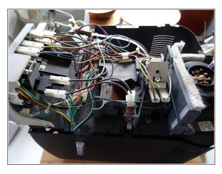
• It's safer to number the cable connectors on the electronics. You probably just need to disconnect the slightly hidden # 14 connector on the two green cables at the very bottom and # 7 on the blue cable on the top.
