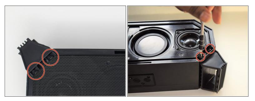
• Remove the 4 7.8mm Phillips screws on the speaker cover using the PH0 screwdriver.
