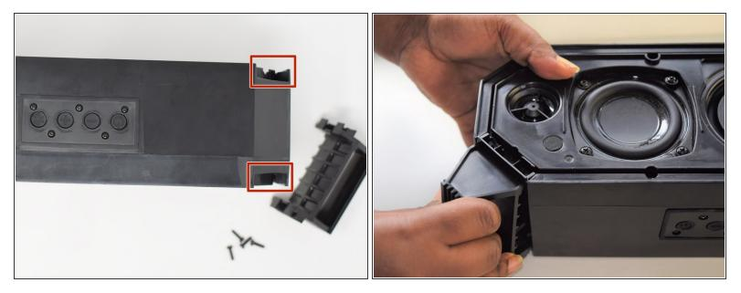
• Carefully slide the handle off the speaker but pushing upwards to the direction the handle is facing.
