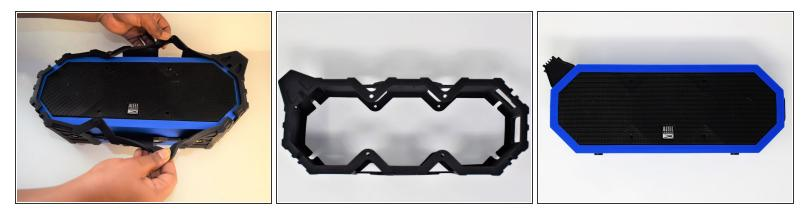
• Remove the outer black rubber housing of the speaker.
