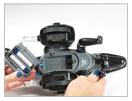
• Remove the battery from the device.
