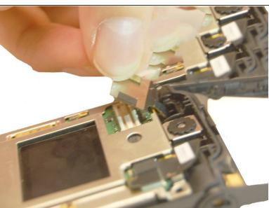
Pull the flex cable connection away from the top of the phone.
