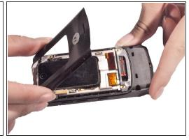
Use a flathead screwdriver or plastic opening tools to help pry the top cover away from the phone.
