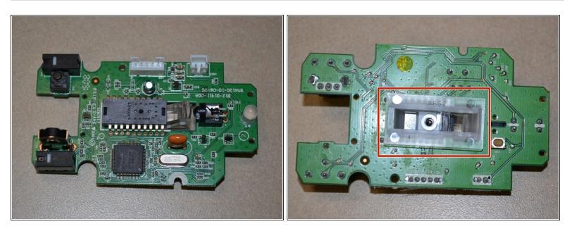
Flip the motherboard over and remove the clear plastic cover from the bottom of the board.
