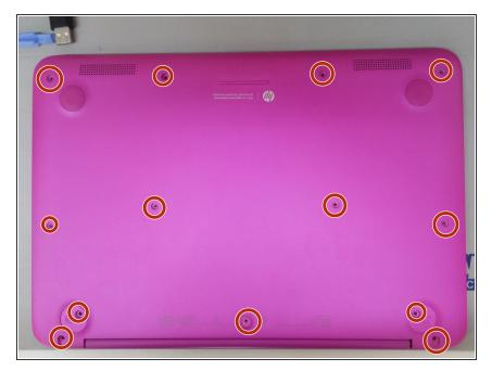
Unscrew all the screws on the back of the laptop and remove the cover
