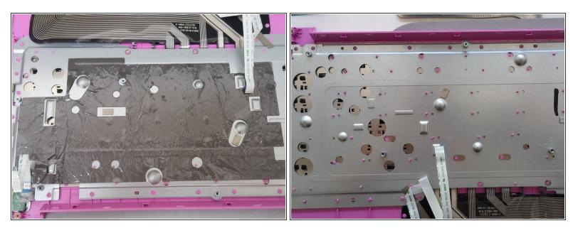
Remove the black adhesive to expose plastic rivets.
