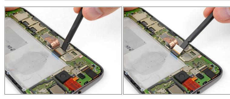
Use your spudger to disconnect the display by prying its connector straight up from the motherboard, on the edge nearest the side of the phone.
