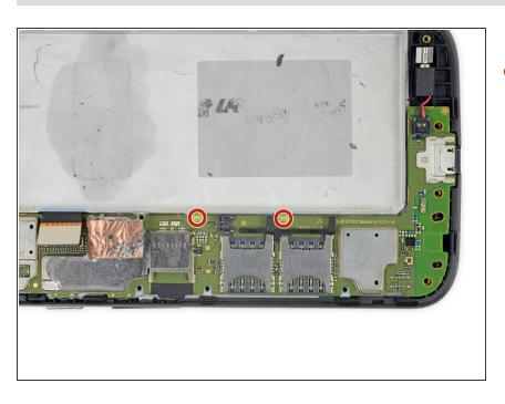
Use a T3 Torx driver to remove the two bronze-colored, 2.4 mm screws securing the motherboard.
