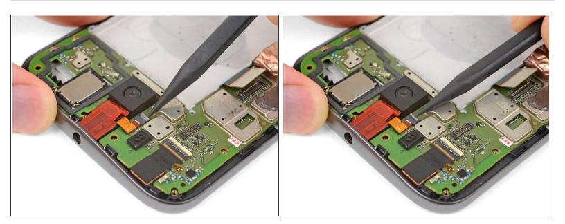
Pry up with your spudger to flip open the locking flap on the headphone jack's <u>ZIF connector</u>.
