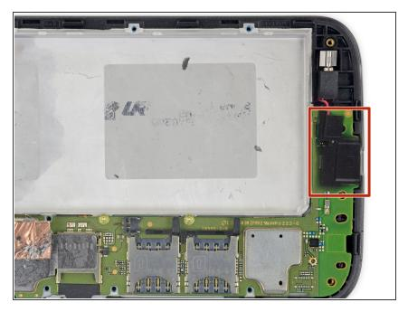
Peel up and remove the black rubber cover from the charging port and vibration motor connector.
