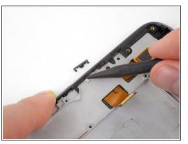
Push the power button out of the frame from the inside by carefully pressing the tip of your spudger against the tops of the two mushroom pins securing it.
