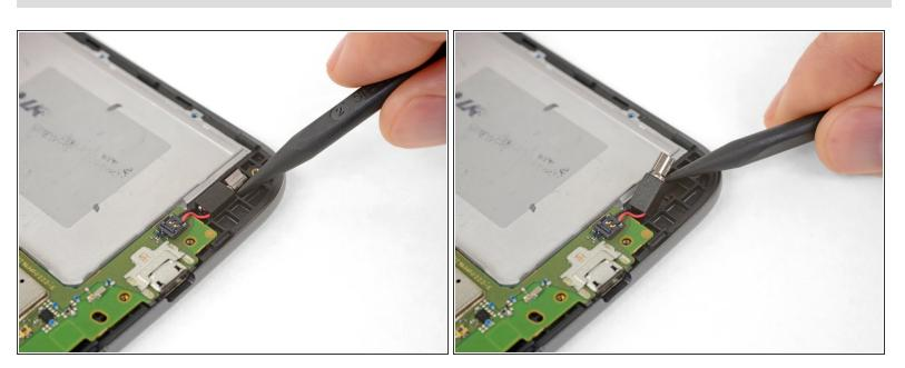
Insert the point of your spudger underneath the vibration motor, and gently pry up to separate it from the frame.
