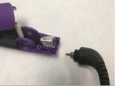
Pull upwards while pulling outwards to disconnect the wire from the housing.
