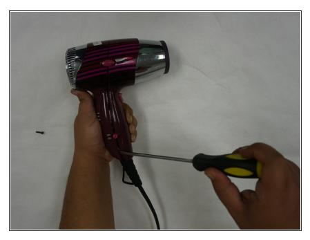
Using a medium flathead screwdriver or better yet iFixit plastic opening tools, gently pry apart the handle from the power cord.
