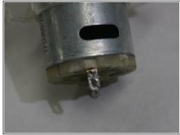
The fan/motor assembly is connected to the heating element assembly at two points need to be desoldered. After pulling the attached wires through the holes the fan/motor assembly will be free from the heating element assembly. Congratulations you have now completely removed the fan/motor assembly from this hair dryer!
