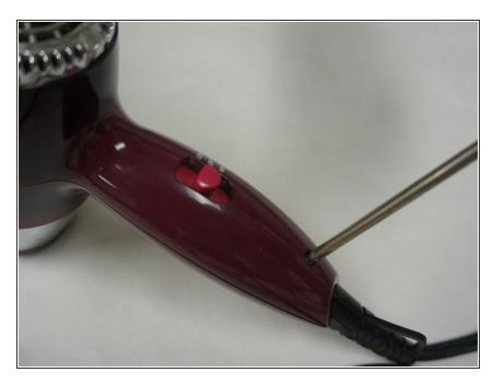
Using a Phillips #3 screwdriver, remove the single 25 mm Phillips head screw in the handle by turning it counterclockwise.
