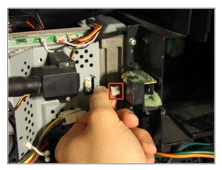
Disconnect the back panel detection sensor by pressing down the white tab and pulling out the connection.
