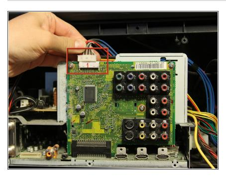
Remove the connection to the front input/output wires by pressing down the white tab and gently pulling up.
