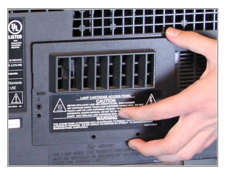
Pull the lamp access panel off of the back panel of the television by pulling straight back on the left side of the panel near the screw then pulling to the left.
