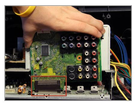
Disconnect the input/output board from the port in the main board by gently lifting upward and pull it out from the casing.
