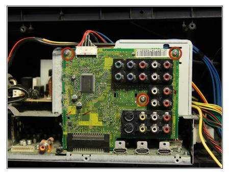
Remove three 10 mm silver, coarse thread Phillips #1 screws holding the input/output board to the case.
