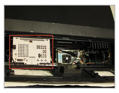
Removing the back panel exposes the input/output board cover plate.
