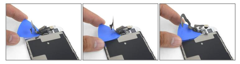
• Slide an opening pick underneath front camera cable assembly, separating the adhesive holding the camera and sensor cable.
