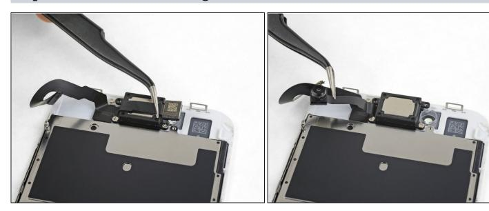
• Lift the front facing camera up out of its socket and swing it out of the way.
