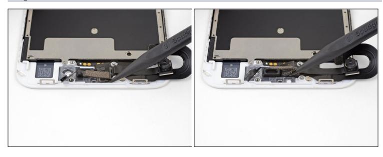
• Slide the tip of a spudger underneath the ambient light sensor flex cable, and lift the sensor out of its housing.
