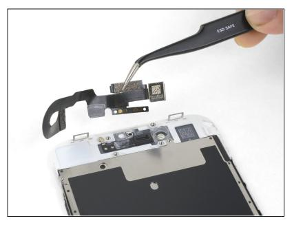
Remove the front camera and sensor cable.
