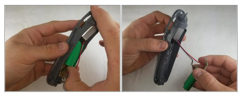
• Remove the circuit board assembly from the frame.
