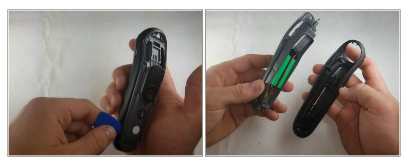
• Use the opening pick to lift the grey frame from the black casing.
