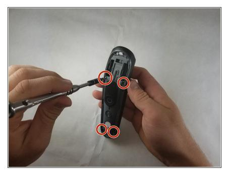
Remove the four 7.0mm Torx T6 screws attaching the grey plastic frame to the black plastic casing.
