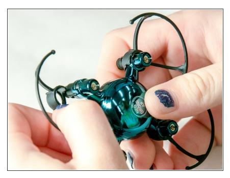
Remove the blade guards by pushing the guards downward towards the padded feet.
