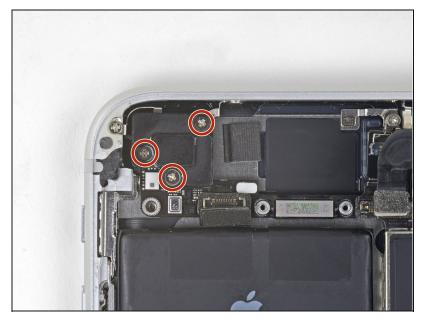
• Remove the three Phillips 1.3 mm screws securing the top left antenna component.
