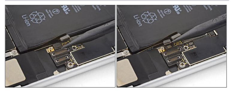
• Use the point of a spudger to pry up and disconnect the Wi-Fi diversity antenna cable.
