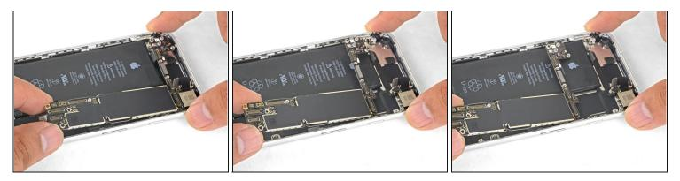
• Grasping it by the edges, lift the logic board near the battery connector and remove it.
