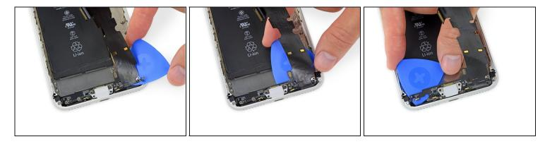
• Slide your pick across the width of the iPhone to separate all the remaining areas of the Lightning connector assembly from the rear case.
