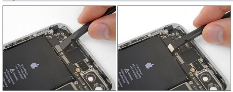
• Prying from the top edge, use your fingernail or a spudger to pry up and disconnect the upper cable connector.
