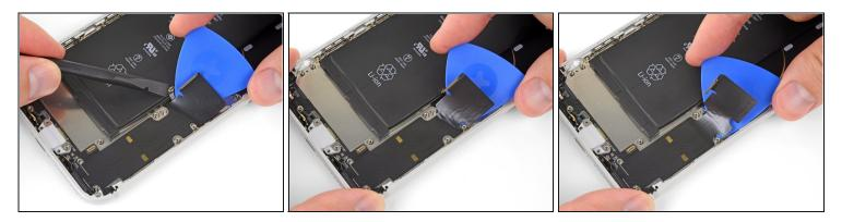
Continue separating the upper portion of the Lightning connector flex cable, being careful not to damage any other components along the way.
