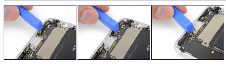
• Use the sharp edge of an iFixit Opening Tool to pry the two microphones free from the adhesive securing them to the lower edge of the iPhone.
