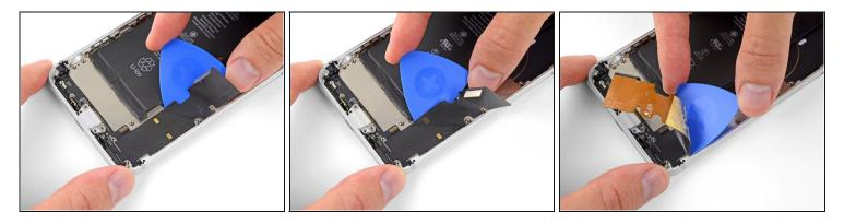
• Continue separating the Lightning connector assembly's flex cable until you pass the lower edge of the battery.
