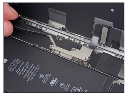
• Remove the lower display cable bracket.
