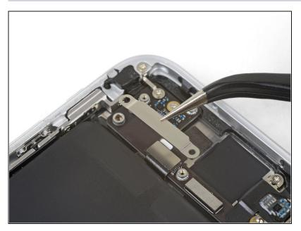
• Remove the upper cable connector bracket.
