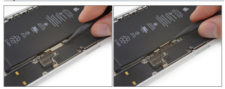
• Use the point of a spudger to pry up and disconnect the Lightning connector assembly's flex cable from the logic board.
