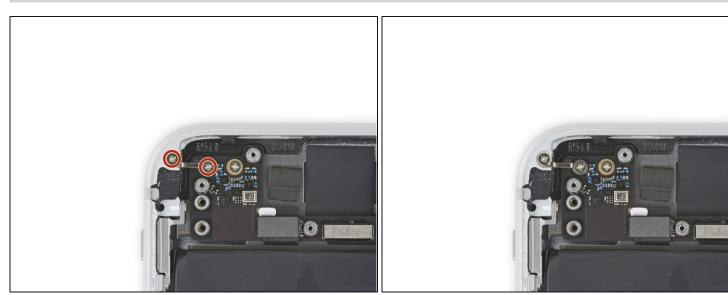
Remove the two 1.2 mm Phillips screws securing the grounding clip at the top left edge of the logic board.
