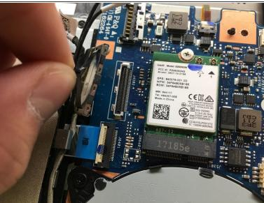
Pull straight up to disconnect the SATA combo cable from the motherboard.
