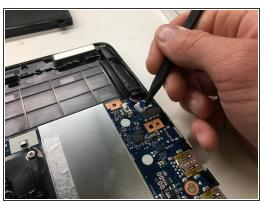
Use a Spudger to push the left speaker cable out the connector.
