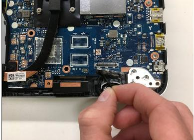
Pull straight up to disconnect the display cable
