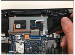
Use a spudger to flip up the retaining flap on the trackpad ribbon cable ZIP socket.
