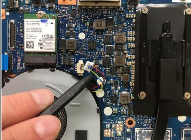
Use the tip of spudger to push out the fan connector.
