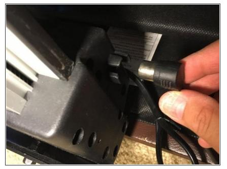
• Disconnect 5-prong plug from the motor unit by pulling it straight up and away from the 5-prong connector on the motor.
