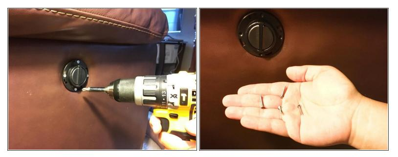
Remove the four 25.4 mm (or 1 inch) Philips #2 screws using a standard Philips #2 screwdriver or a power drill with a Philips #2 screwdriver bit.
