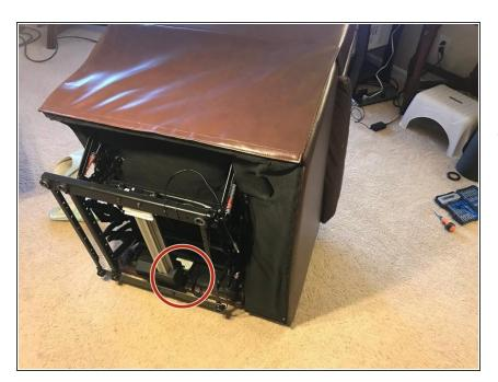
• Lean the recliner over to expose the 5-prong plug that is at one end of the power switch cable and is also connected to the recliner motor.
