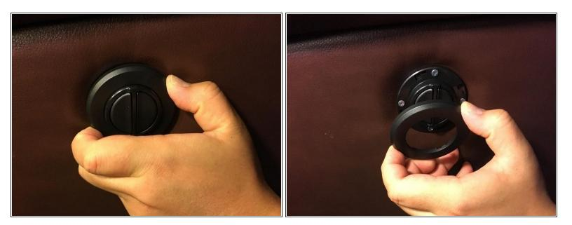
Apply pressure by pushing in and turning the screw cover in a counter-clockwise direction in order to remove the cover and expose the screws holding the round power switch to the recliner's housing for the switch.
