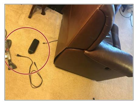
Disconnect the power supply, power adapters, surge protectors, power strip and wall plug from the wall outlet.
