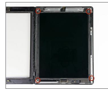
• Remove the four 2 mm Phillips #00 screws securing the LCD to the aluminum frame.
