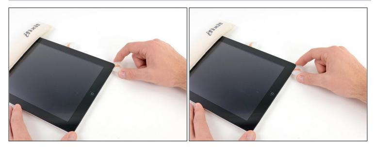
• Slide the opening pick around the bottom right corner of the iPad, releasing the adhesive there.
