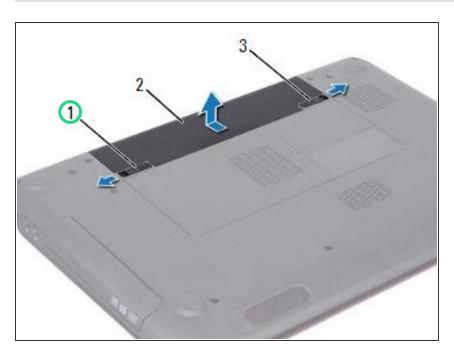
Slide the battery release latch and the battery lock latch to the unlock positions.
