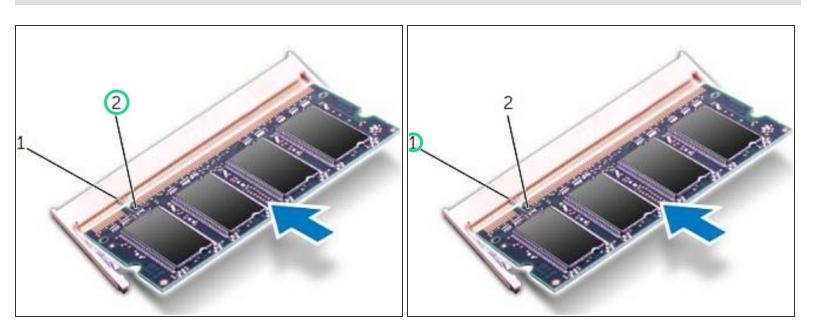
Align the notch on the memory module with the tab on the memory-module connector.
