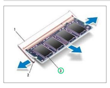
Slide the memory module firmly into the slot at a 45-degree angle, and press the memory module down
