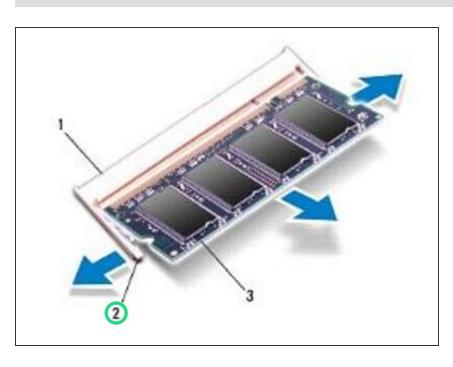
Use your fingertips to carefully spread apart the securing clips on each end of the memory module connector until the module pops up.
