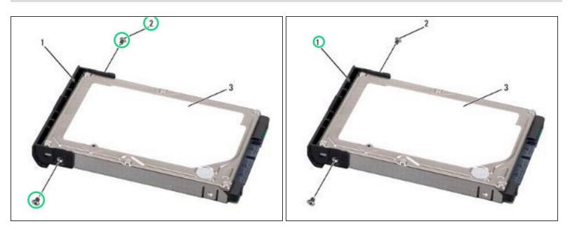
Remove the two screws (one from each side of the hard drive cover), then pull to separate the cover from the hard drive.
