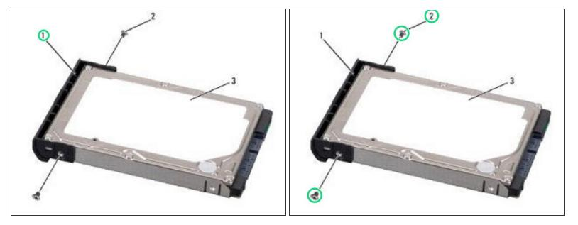
Replace the hard drive cover and tighten the two screws to secure the cover to the NEW hard drive.
