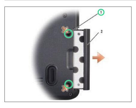
Replace the two screws to secure the hard drive.
