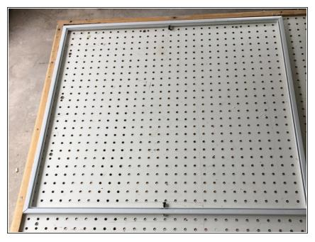
Make sure you start with a frame thats straight and square. I use a table with cleats at 90 degrees to make sure each frame is correct
