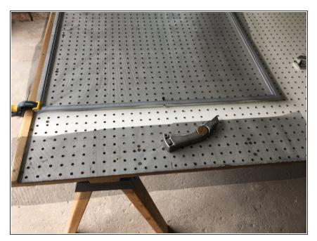
• Trim off the excess leaving about 2 inches over the frame before rolling the material in. Leaving too much material hanging will prevent the cloth from laying flat and square.
