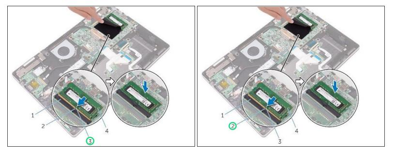
Align the notch on the NEW memory module with the tab on the memory-module slot.
