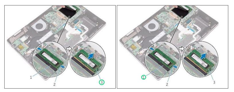
Remove the memory module from the memory-module slot.
