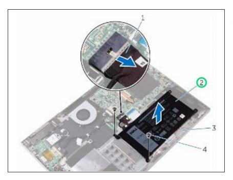
Lift the battery along with its cable off the palm rest and keyboard assembly.
