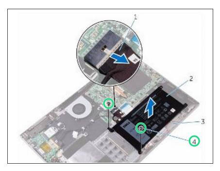
Replace the screws that secure the battery to the palm rest and keyboard assembly.
