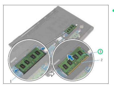
• Remove the memory module from the memory-module slot.
