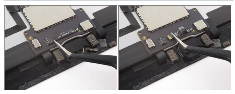
• Use tweezers to slide the cable out of the ZIF connector.
