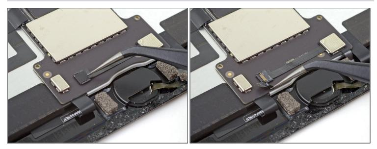
• Use <u>tweezers</u> to remove the tape covering the ZIF connector above the home button.
