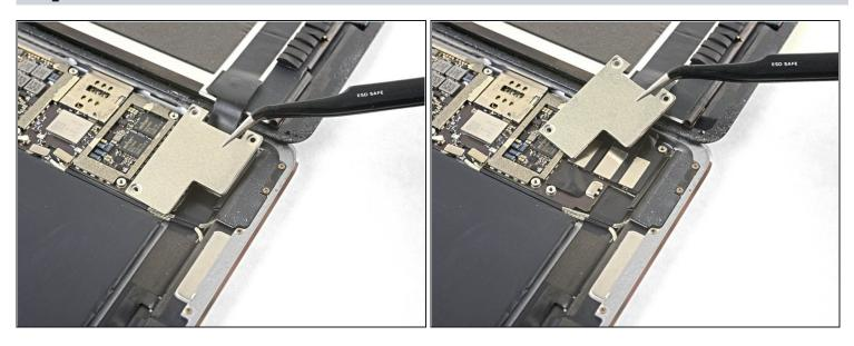
• Remove the display cable bracket.
