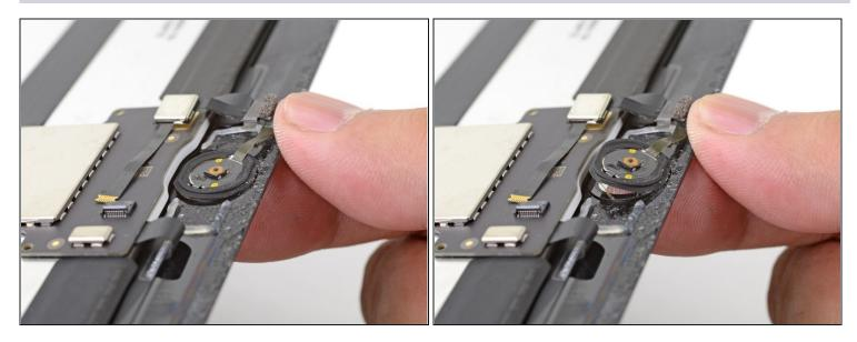
• Gently push the home button from the front of the display inward using the tip of a finger.
