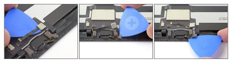
• Starting from the ZIF connector, use an opening pick to separate the home button cable from the adhesive holding it in place. Stop when you reach the home button.
