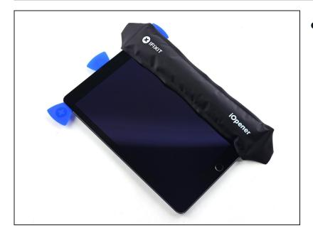
• Reheat the iOpener and lay it over the right edge of the display to loosen the adhesive underneath.
