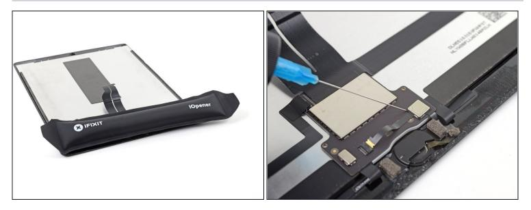
The home button's ribbon cable is **very** fragile. If it gets damaged, Touch ID will no longer function.
