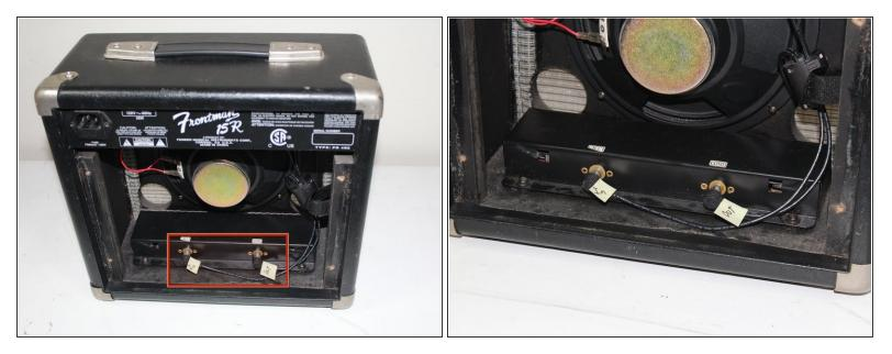
There will be two black wires connecting the top mounting bracket to the reverb box at the bottom
