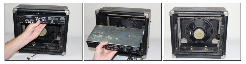
• Pull the mounting bracket free from the frame. It may be wedged in very snug, in which case, use a plastic opening tool/spudger to pry it loose from the front.
