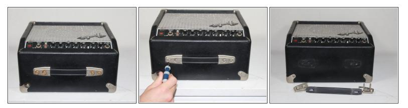
Use a Phillips #1 screwdriver to unscrew the four 36.4 mm screws holding the mounting bracket to the top of the amp.
