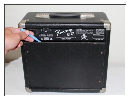
Once the screws are out, use a plastic opening tool or spudger to pry the top of the back panel open. There may be some resistance, but it will eventually pry loose.
