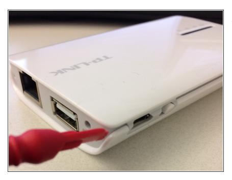
First, open the case by prying off the bottom the same way you access the battery. Use a thumbnail on this side and the other side
