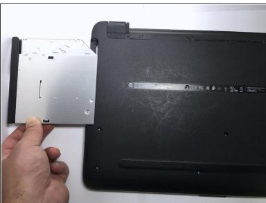
Use prying tool to remove optical drive
