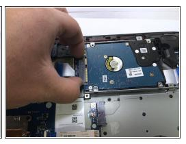
Use spudger to loosen the SATA connector then disconnect the cable and remove the hard drive.
