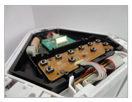
If the button sheet or button is damaged, you may need to purchase a new button sheet to replace the damaged one.
