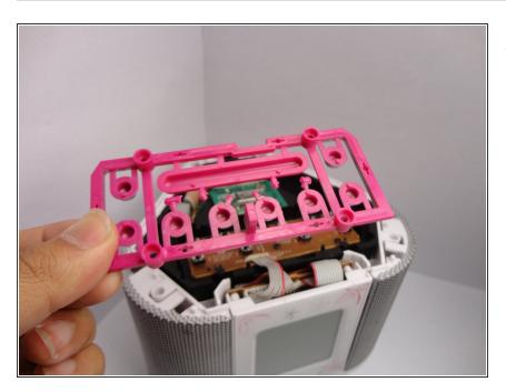
Examine the button sheet to check for any damages that may prevent the buttons from working.
