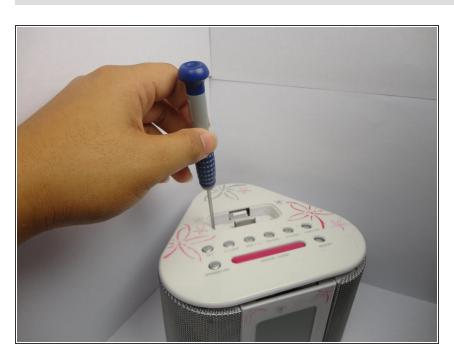
Unscrew the screws on the top side of the device.
