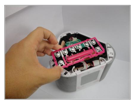
Remove the button sheet off of the device.
