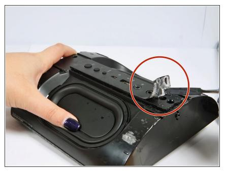
Using the metal spudger, peel the backing off of the back panel of the speaker to reveal 4 screw holes.
