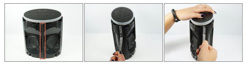
• Peel off all rubber strips along sides, middle front and middle back of the device.
