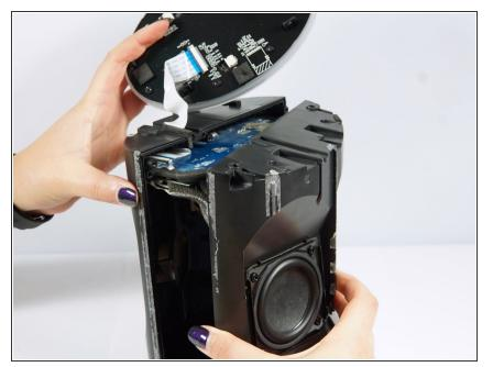
Pry apart the two sides carefully. The halves will not be able to separate completely because of wires and the motherboard.
