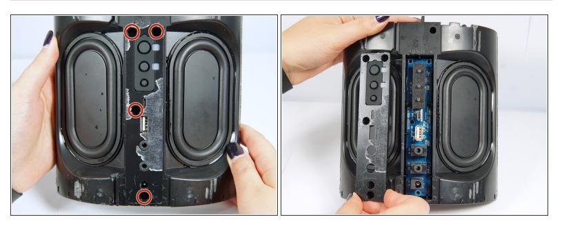
Remove the four 4 mm screws with a Phillips #2 screwdriver, then lift off the panel.
