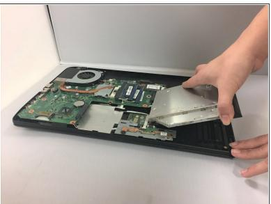
Grab hold of the optical drive and elevate it slightly and remove it from the computer.
