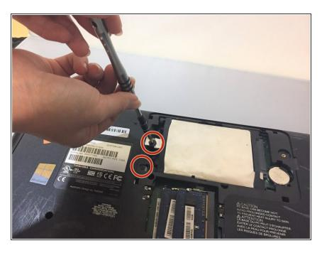
Using the Phillips #1 screwdriver, remove the two screws holding the hard drive in place.
