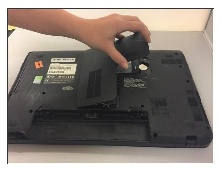
Remove the middle plastic cover to expose the hard drive.
