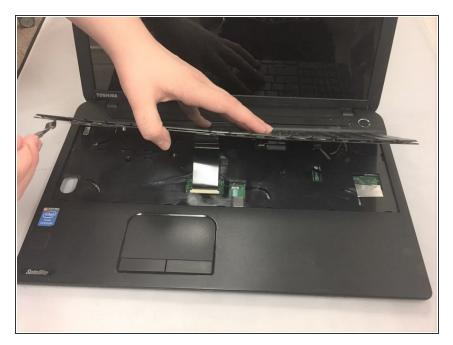
Using the metal spudger, carefully pry up the edges of the keyboard.
