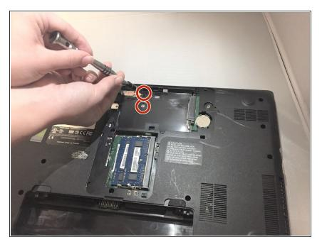
Use the Phillips #1 screwdriver to remove the two screws under the hard drive.
