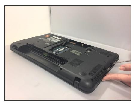
Use a metal spudger and run it along the edges of the computer to take off the plastic back cover.
