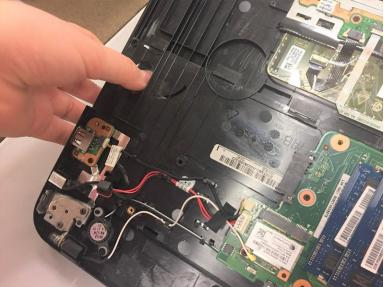
Using your thumb, apply a light amount of pressure to the underside of the keyboard until it pops out a bit.
